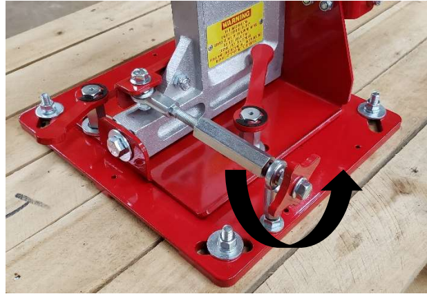
Figure 3: Counterclockwise rotation moves target path to the right.
