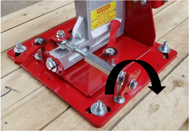
Figure 2: Clockwise rotation moves target path to the left.
