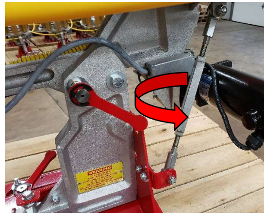
Figure 5: Rotation moves target path down.
